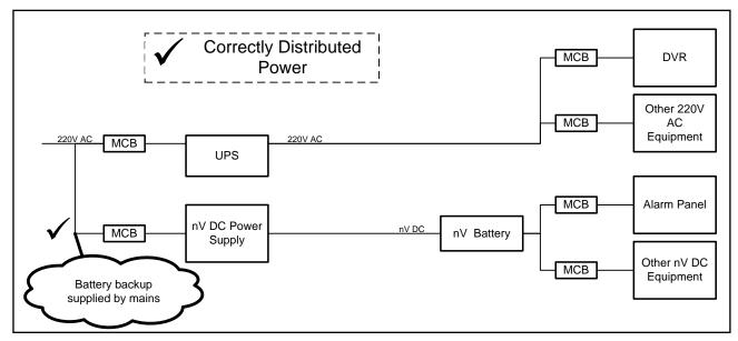
Figure 11: Correctly Distributed Option 2 Power, Battery Parallel to UPS
