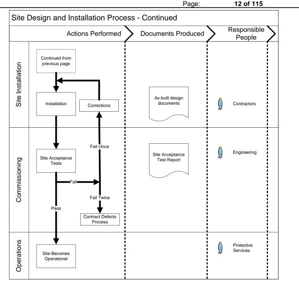
Figure 2: Design and Installation Process (pg2)
