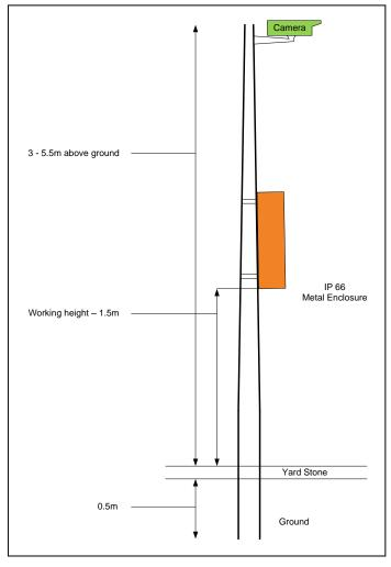
Figure 15: Camera and Metal Enclosure Mounted on Concrete Pole
