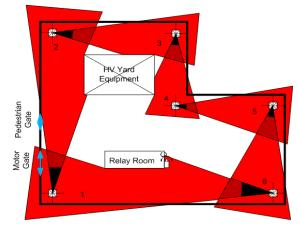
Layout and Arrangement of Perimeter Camera System bundled with Intelligent Video Analytics for Detection. Irregular shape site  $\,$  – Option2
