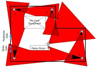
Layout and Arrangement of Perimeter Camera System bundled with Intelligent Video Analytics for Detection. Irregular shape site – Option 3
