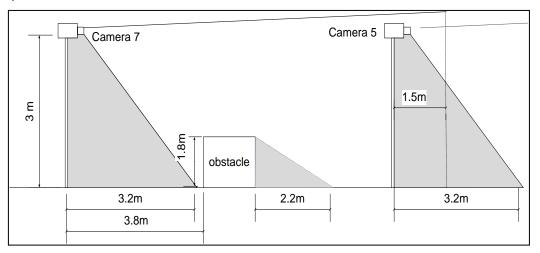
Figure 24: Example of Measured Vertical Field of View of a Camera
