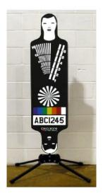
Figure D.1: Rotakin Test Target
