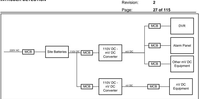
Figure 9: Preferred Power Distribution, Using Backup Power from the Site
