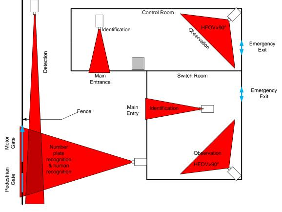
Figure 3: Example of Camera Placement, FOV and Purpose
